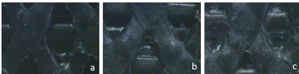
Figure 1. Optical microscopy images of the 3D printed membrane surface with a) one, b) two and c) three layers of PVA.
