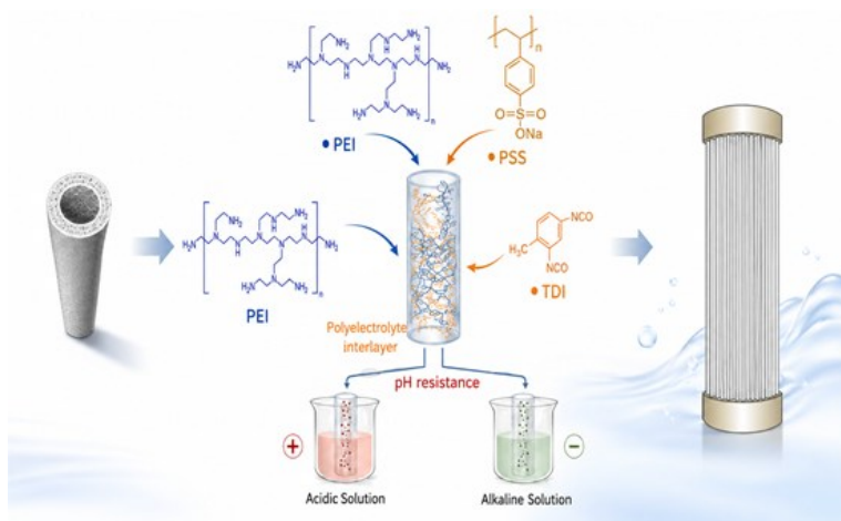
Figure 1. Polyelectrolytes-assist IP in the preparation of scalable, high-performance acid and alkali resistant polyurea membranes.
